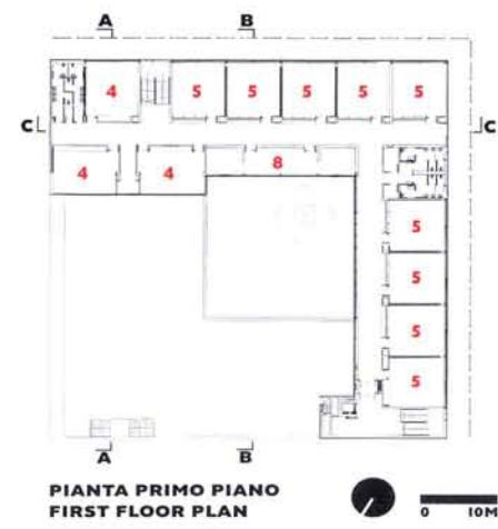
**IL PROGETTO APPLICA PRINCIPI BIOCLIMATICI E DI RISCALDAMENTO PASSIVO: GRAZIE AL TETTO VERDE, ALL'ORIENTAMENTO SOLARE E ALL'UTILIZZO DI SONDE GEOTERMICHE PER RISCALDARE LA PALESTRA, LA SCUOLA HA UN CONSUMO ANNUO PARI A 3,6 KW/H/M<sup>2</sup> (CLASSE A+ DI CASACLIMA). IL MURO DELLE AULE, REALIZZATO IN LEGNO, OSPITA AL SUO INTERNO UNA PICCOLA BIBLIOTECA; VERSO IL CORRIDOIO, FUNZIONA COME APPENDIABITI. LE PANCHE, DURANTE LE ATTIVITÀ SPECIALI, POSSONO ESSERE SPOSTATE NEGLI SPAZI COMUNI.**
